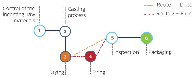
Our products can be delivered dried or fired. The dried ones are refractories which had had a thermal treatment that can warranty no free and chemical water into the microstructure. On the other hand, fired products had been fired at high temperatures, allowing the ceramic bond development which improves refractory properties. The selection between a dried and a fired product should be made taking into account process conditions and also, the properties of the materials.
